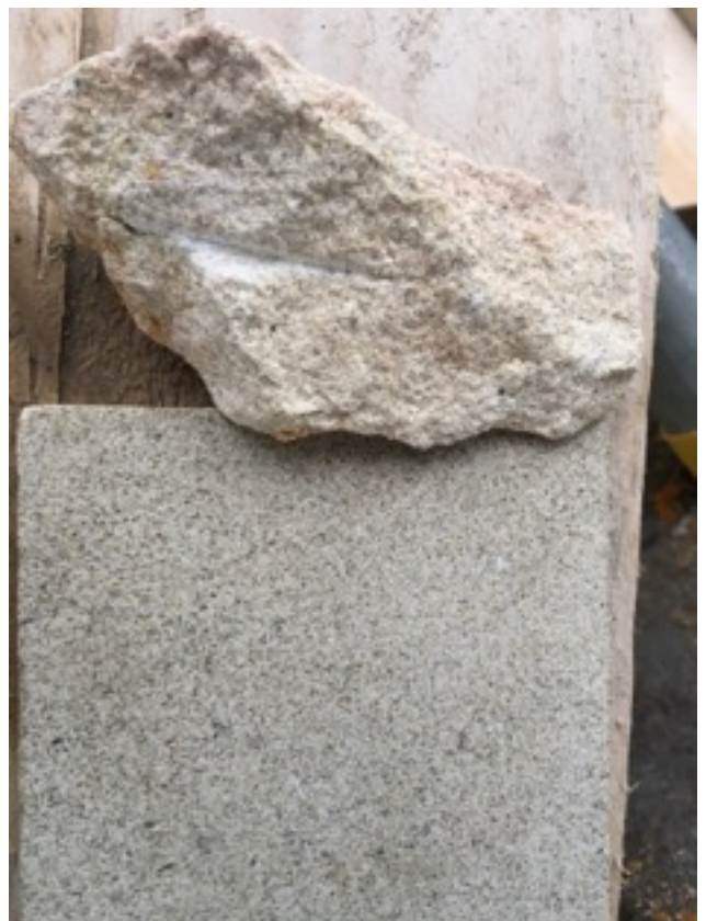
Sample of Crosland Hill sandstone, (grey/ buff ) adjacent to piece of freshly broken existing stone
